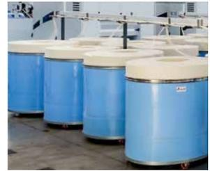
The 43% longer runtimes of the JUMBO CANS in the creel results in reduced downtimes on autoleveller draw frames or lap winders.
