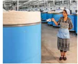
Even fully loaded – with up to 83 kg card sliver – the JUMBO CANS can be moved very easily over straight hall floors.
